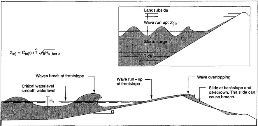
Figure 6. Design of dike height.
