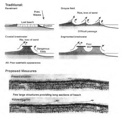
Figure 4 Performance of traditional coast protection measures and proposed upgrading to shore protection scheme for moderate/exposed coasts with small angle of incidence.
