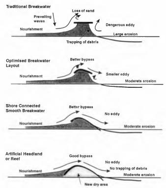
Figure 5 Optimisation of coastal breakwater to artificial headland, applicable for moderate/exposed coasts for small angles of incidence.
