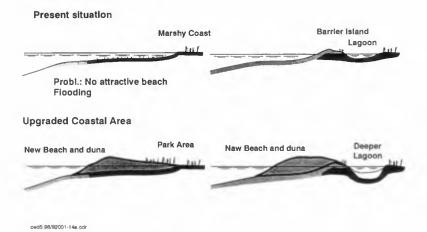
Figure 3 Upgrading of: (a) Protected coastal areas with all directions of wave approach, coastal types 1P – 4P and (b) Moderate/exposed beaches with perpendicular wave approach, coastal types 1M and 1E.
