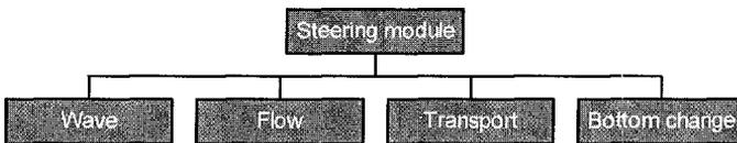
The model structure consists of a steering module and four computational modules, as outlined in Figure 1. The steering module calls the computational modules in any prescribed order, and arranges the time-progress of each module. It allows iterations between modules. The computational modules are:
