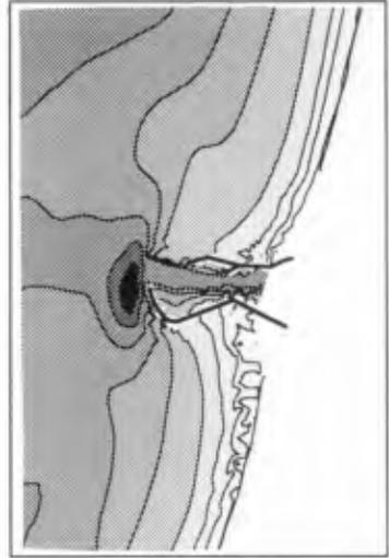
Figure 15. Computed 1976 bathymetry
