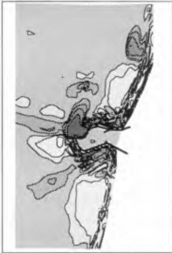
Figure 7. MOR with wave stirring, '68-'73, roughness 5 cm..
