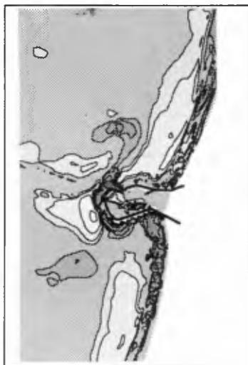
Figure 13. Depth changes '68-'76, simulation including cross-shore transport and dredging.
