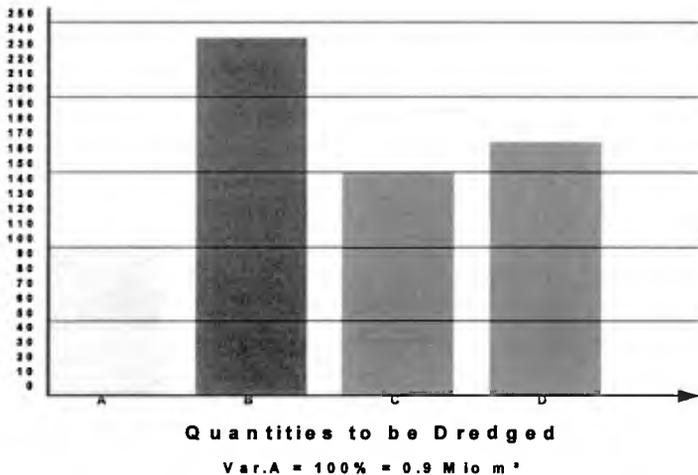
Fig. 14 Quantities of Dredged Spoil for Alternatives A - D
