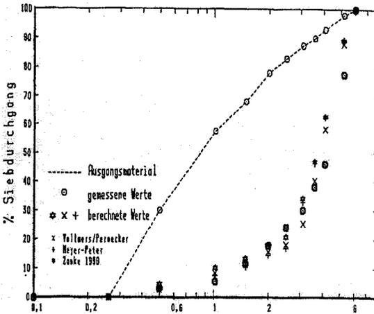
Fig. 6: Comparison between measured and calculated sediment transport
