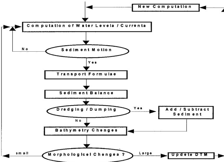
**Fig. 7 Computational Steps for the Morphodynamic Model**
