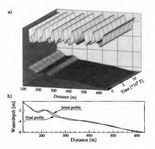
Figure 7: Prediction of changes from the typical two-bar system by moderate summer storms (with  $T_p = 10$ s): (a) temporal evolution to a one-bar system from the typical two-bar profile, (b) initial and final profiles from (a).
