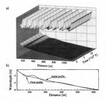
Figure 4: Prediction of the formation of the typical two-bar system by major storms (with  $T_p = 15s$ ) at Duck, NC: (a) temporal evolution of the bar system from the featureless equilibrium profile, (b) initial and final profiles from (a).
