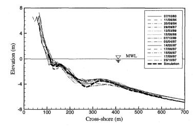
Figure 11: Prediction (heavy dashed line) and observations of episodic, nonstationary behavior of the two-bar system at Duck, NC.
