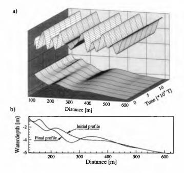
Figure 10: Prediction of an episodic change in the two-bar system at Duck, NC (a) migration of the post-storm profile under extreme waves  $(T_p = 15 \text{ s})$ , accompanied by a 1.2-m surge above the mean water level, (b) initial and final bed profiles from (a).
