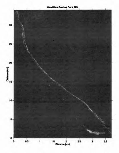
Figure 4. Example 35 second aerial time-exposure along 33 km of the North Carolina coast just south of Duck. The coordinate system (in km) has arbitrary origin with north towards the top and ocean (east) to the right in the image. The image resolution is 5 m in both the cross- and along-image axes. The sand bar is located very close to shore, with no discernible offshore breaking apparent seaward of about 80 m from the shoreline.
