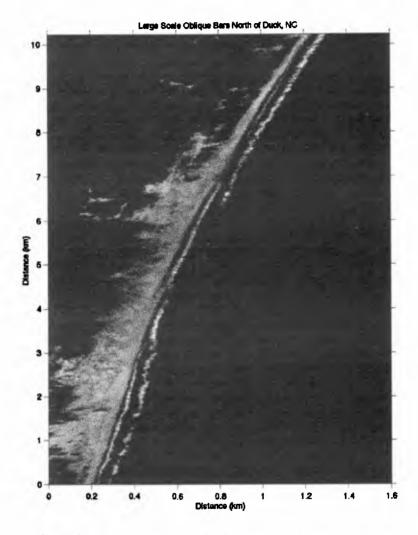
Figure 2. Example 35 second aerial time-exposure along 11 km of the North Carolina coast just north of Duck. The coordinate system (in km) has arbitrary origin with north towards the top and ocean (east) to the right in the image. The image resolution is 5 m in both the cross- and along-image axes. The location of large scale oblique sand bars are indicated by the white bands located 25-200 m offshore.
