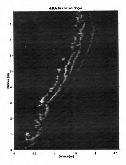
Figure 6. Example 35 second aerial time-exposure along 9 km of the northern Oregon coast near Tillamook Bay. The coordinate system (in km) has arbitrary origin with north towards the top and ocean (west) to the left in the image. The image resolution is 5 m in both the cross- and along-image axes. The large scale nearshore morphology shows long, sinuous bar features which sometimes attach to the shoreline.
