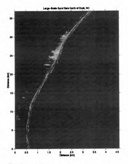
**Figure 3.** Example 35 second aerial time-exposure along 36 km of the North Carolina coast just north of Duck. The coordinate system (in km) has arbitrary origin with north towards the top and ocean (east) to the right in the image. The image resolution is 5 m in both the cross- and along-image axes. Several oblique sand bars emanating away from the coast are visible in the image as the white bands with 25-200 m of the shoreline.
