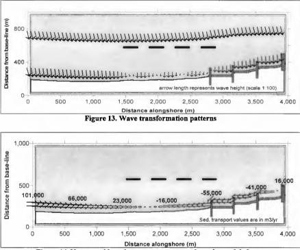
Figure 14. Net annual longshore transport rates along the modeled area
