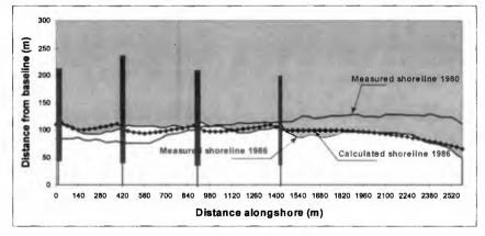
Figure 6. Model calibration results
