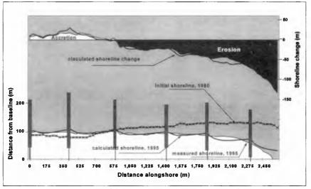
Figure 7. Sea Isle City model verification and final results
