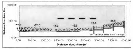
Figure 15. Net annual cross-shore sediment transport along the modeled area
