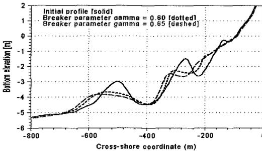
Fig. 3: Effect of breaker parameter  $\gamma$  on final profile evolution
