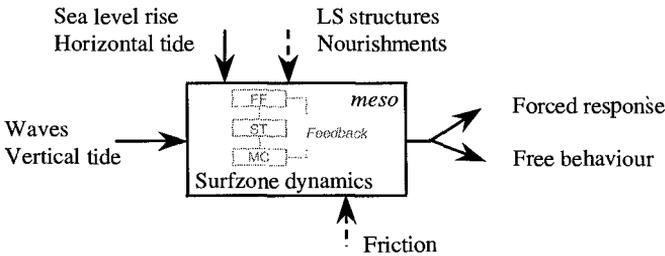
Fig. 2: Schematization of a meso-scale coastal system
