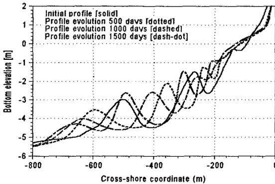
Fig. 6: Bar behaviour in calibrated model
