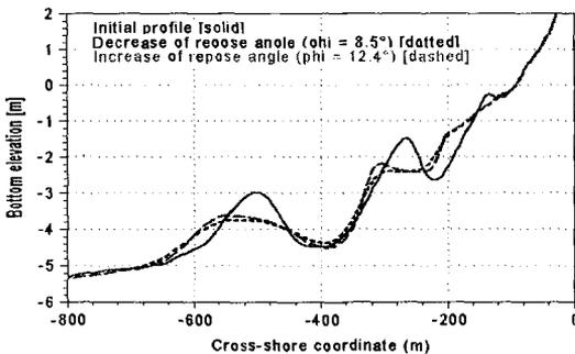
Fig. 5: The effect of  $\tan(\phi)$  on final profile evolution
