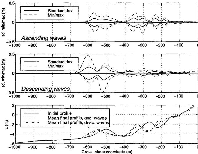
Fig. 8: Variability in final profile evolution in case of sorted wave height input
