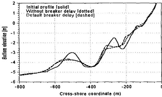
Fig. 4: Effect of breaker delay on final profile evolution
