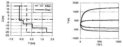
In Figure 3 as an illustration, the cross-shore evolution is given for an initially steep cross-shore profile using one single wave condition as a forcing agent.
