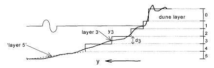
Figure 1: Layer schematization used in the model
