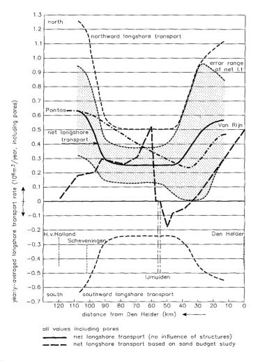
Figure 5: Comparison of computed wave-induced longshore transport [Van Rijn, 1995, 1997].
