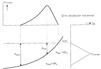
Figure 2: Shematization of wave-induced longshore transport
