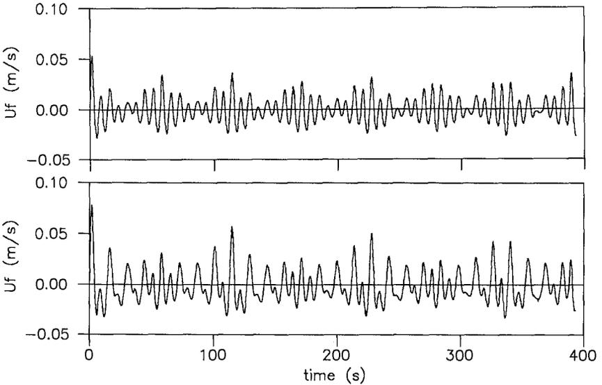
Fig. 10 Instantaneous shear velocities due to different wave groups.
