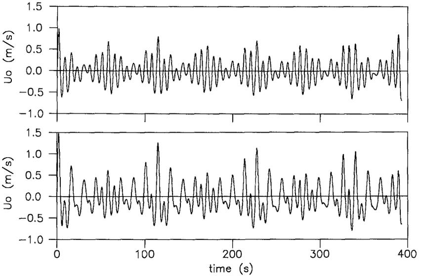
Fig. 9 Instantaneous bed orbital velocities due to different wave groups.
