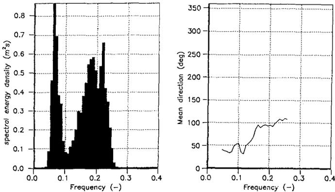
Fig. 3 Typical wave spectrum at Pecém. Two distinct peaks can be observed with frequencies of approximately 0.08 and 0.12  $s^{-1}$  representing swell and wind waves (sea) respectively. The wave directions of the two dominant wave components are varying from approximately 30° N for the swell to approximately 120° N for the sea waves.
