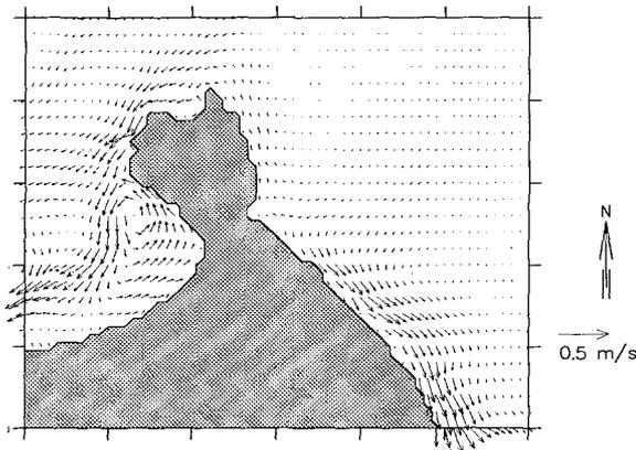
*Fig. 8 Wave driven current around the headland for the present situation (Swell).
