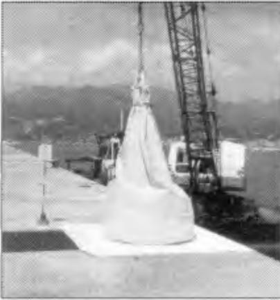
Fig. 1 2 tons sand sac used for caisson excitation.
