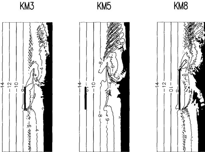
Figure 5. Predicted bathymetry after 10 days of simulation
