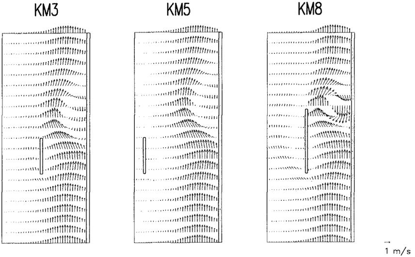
Figure 3. Initial wave-driven current fields
