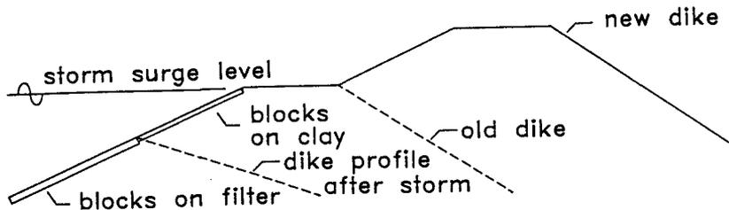
Figure 1 Cross-section of a dike before and after reinforcement
