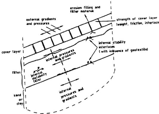
Figure 4 Components of loads and structure
