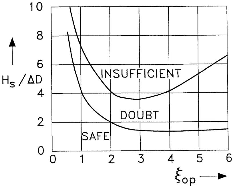
Figure 6 Example of testing graph for top layer stability
