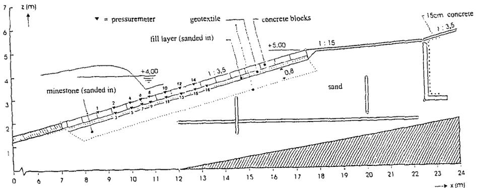
Figure 8 Large scale model test on aged placed block revetment
