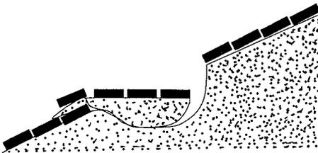
Figure 5 Slide failure of the subsoil
