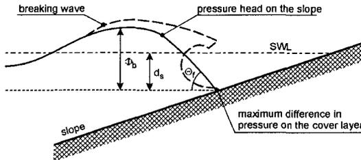
Figure 2 Schematization of pressure head on a slope
