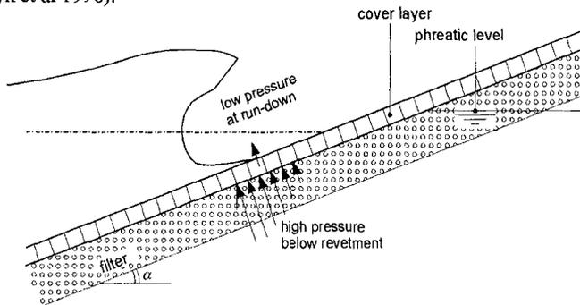
Figure 1, Pressure development in a revetment structure
