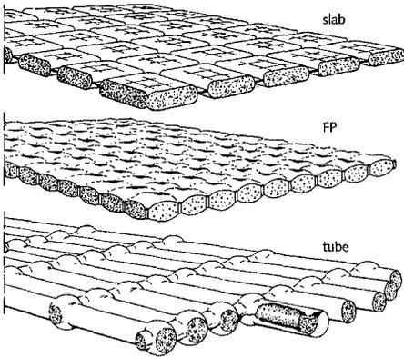
Figure 6 Examples of concrete-filled mattresses
