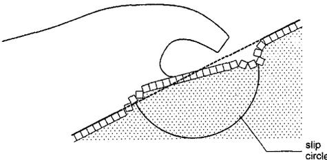
Figure 3 Schematised development of S-profile and possible local sliding in the base (sand)
