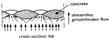
Figure 7, Principles of permeability of Filter Point Mattress
