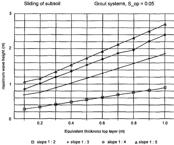
Figure 4, Geotechnical stability, design diagram for grouted systems and  $H_s/L_{op} = 0,05$
