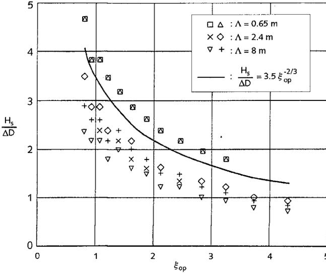
Figure 8 Calculation results for concrete mattresses ( $H_s/\Delta D < 4$  because of acceptable crack distance due to impacts on spans).
