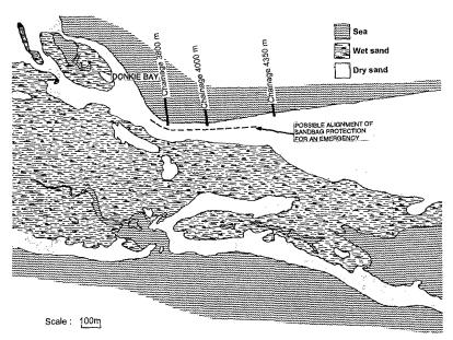
Figure 5: Possible position of the sandbag protection
