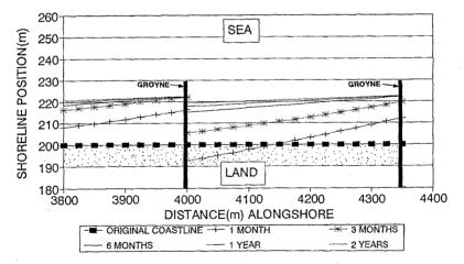
Figure 9: Shoreline evolution caused by two 61 m long groynes
