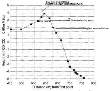
Figure 6: Position of the sandbag protection on the profile
