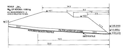
Figure 7: Cross-section of rock berm
