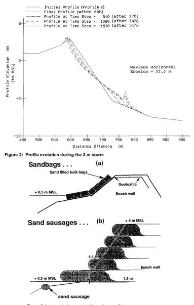
Figure 3: Low-cost shore protection using sandbags and sausages
