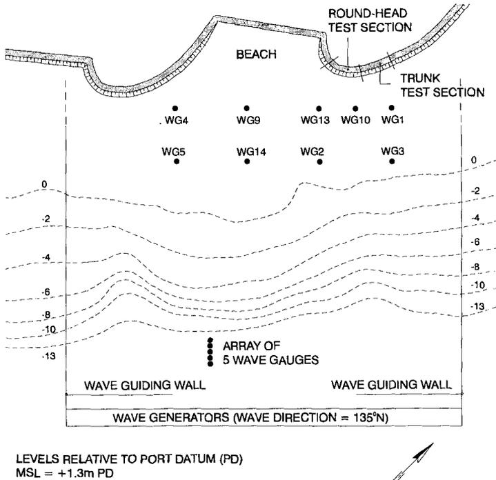
Figure 6. Layout of physical model.
