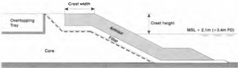
Figure 7. Cross-section of revetment test section.
