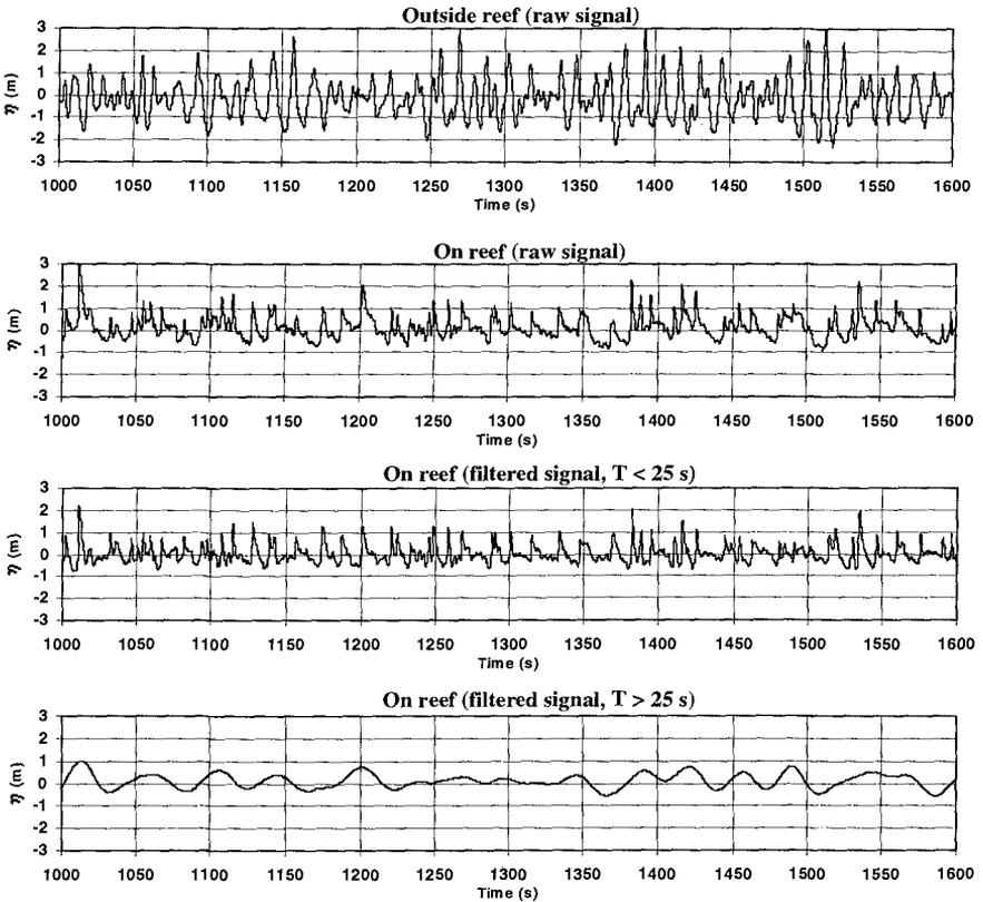
Figure 9. Time series of surface elevations on the reef ( $H_{m0,i} = 4.0$  m,  $T_p = 12.7$  s).
