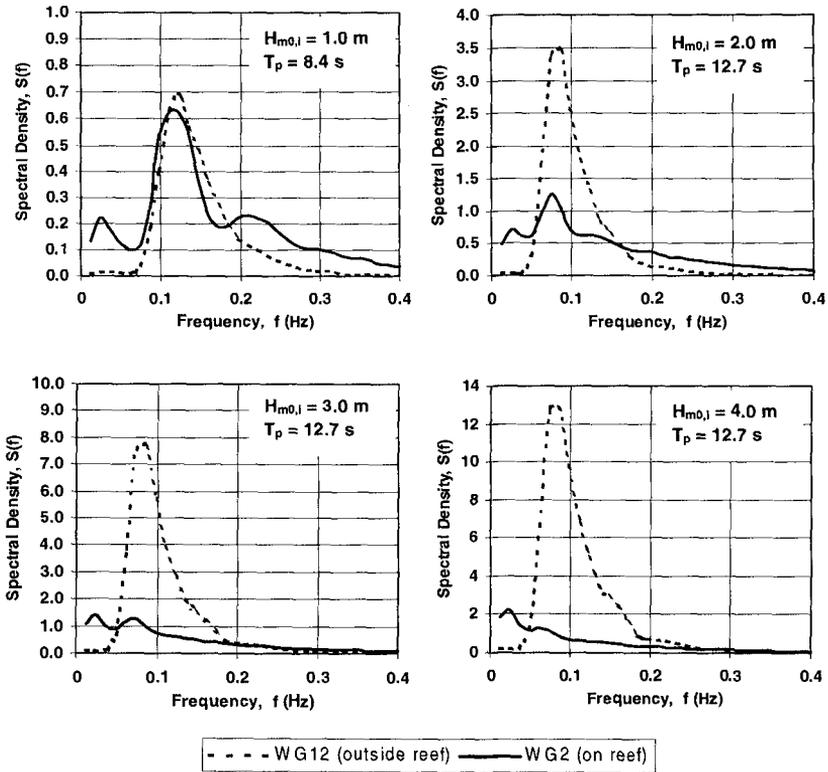
Figure 8. Measured wave spectra on the reef and outside the reef.
