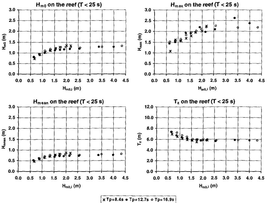
Figure 11. Wave conditions at WG13 on the reef (short-period wave components).
