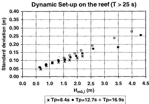
Figure 10. Standard deviation of the dynamic set-up on the reef versus  $H_{m0,i}$ .
