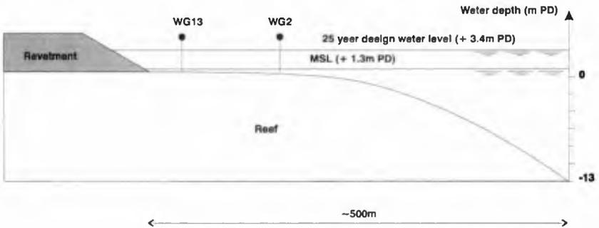
Figure 5. Sketch of a typical cross-section of the reef (distorted length scale).
