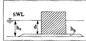
**Low and High Mound Breakwaters (LMB and HMB):** they consist of a rubble mound layer of various thickness and a caisson structure sitting on top of this mound. The relative berm height  $h_b^*$  varies from 0.3 to 0.9. Low mound breakwater (LMB,  $h_b^* = 0.3 \div 0.6$ ) and high mound breakwater (HMB,  $h_b^* = 0.6 \div 0.9$ ) can be distinguished. This type of breakwater can cause severe breaking at the wall and high loads at the structure.
