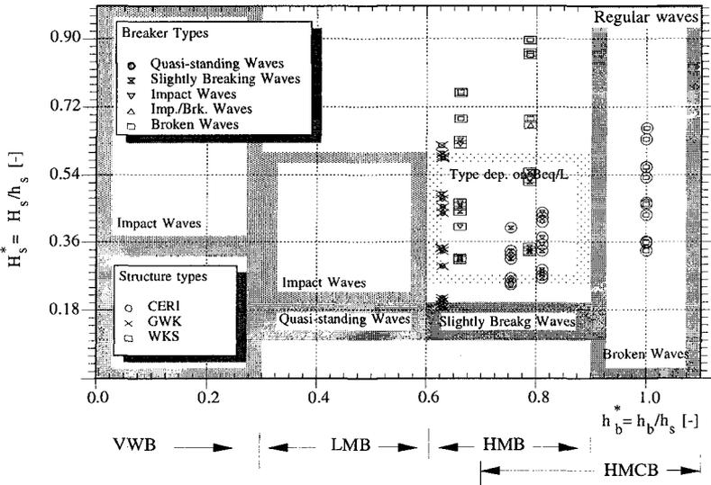
**Figure 9.**  $H_s^*$  vs  $h_b^*$  for Regular Wave Tests (All Data Sets)
