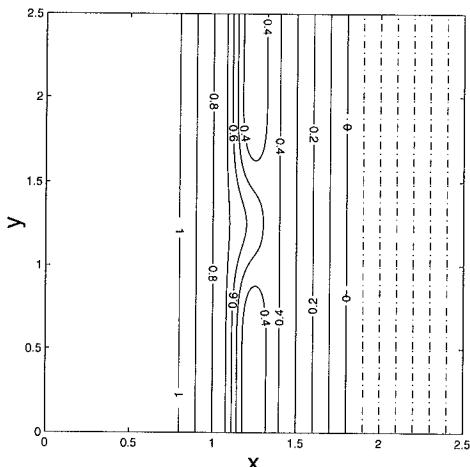
Figure 2: Contour plot of the bed,  $d(x, y)$ . Those above the initial still water level are shown with dashed lines. Contour interval: 0.1.
