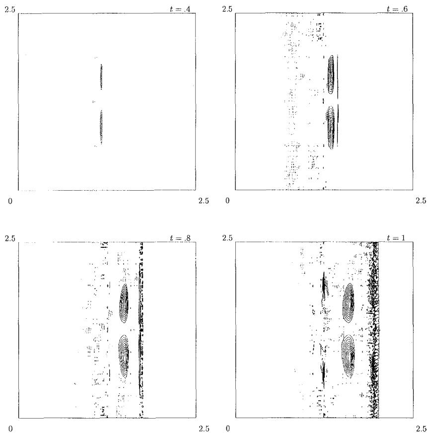
Figure 7: Contours of potential vorticity with 9 contours in  $[-0.3, -0.06]$  and  $[0.06, 0.3]$ .
