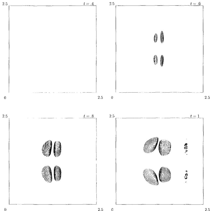
Figure 6: Alongshore velocity component,  $v$ , with 20 contours in  $[-0.03, -0.015]$  and  $[0.015, 0.03]$ .
