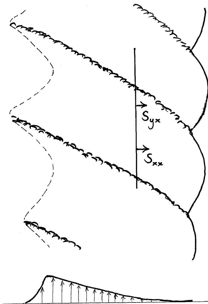
Figure 1. The irregular heavy lines sketch the positions of bores due to regular obliquely incident waves approaching a shoreline on the right. The flux of both x- and y-momentum past a shore-parallel line is indicated by arrows. The dashed line is an estimate of the edge of the region of vorticity as it is displaced by the wave motion. The lower profile is a sketch of a longshore current profile in the absence of horizontal mixing.
