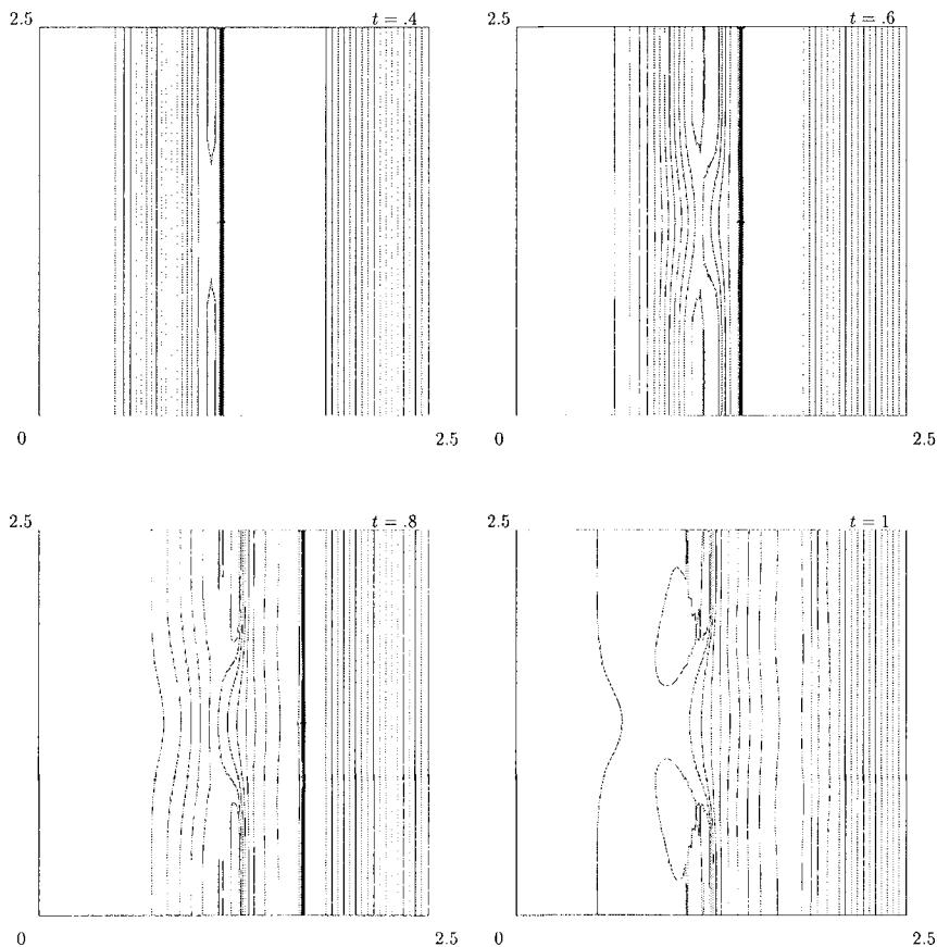
Figure 4: Contours of water surface height,  $h - d$ , with 25 contours in each of the intervals  $[-1.0, -0.04]$  and  $[0.04, 1.0]$ . Contours of the exposed beach are also included.
