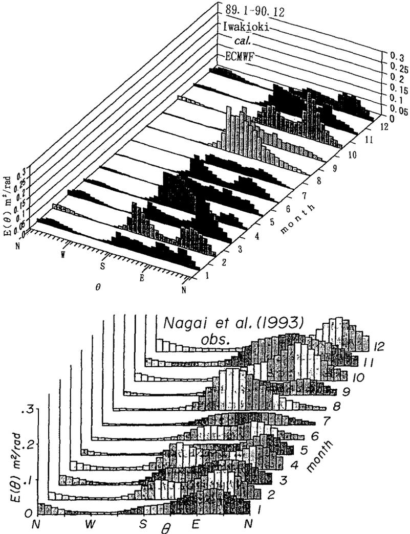
Figure 9. Comparison of Hindcast and Measurement for Monthly-Averaged Directional Energy
