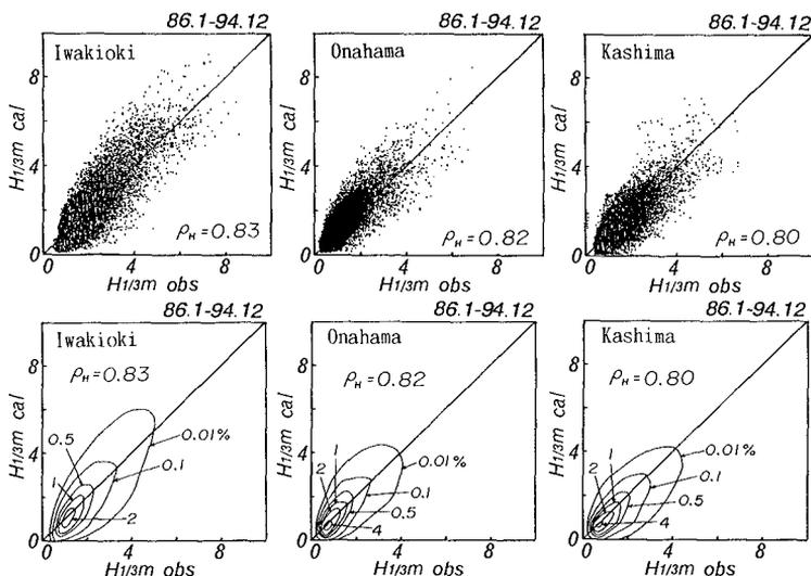
Figure 4. Scatter Diagram between Hindcast and Measurement for Significant Waves and Contour Plot of Relative Occurrence Frequency in a Segment of Wave Height at 3 Stations
