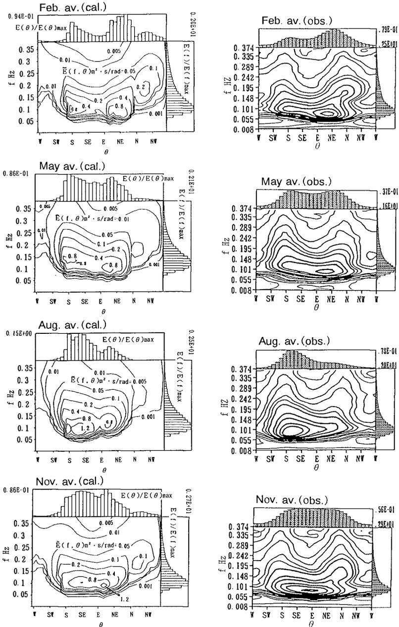
Figure 11. Comparison of Hindcast and Measurement for Monthly-Averaged Directional Spectrum, Directional Energy and Frequency Spectrum
