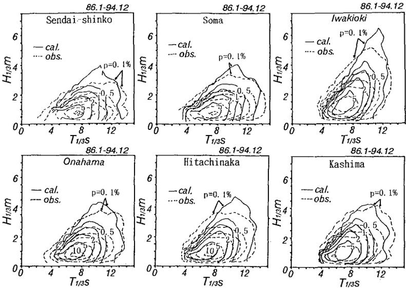
Figure 7. Comparison of Hindcast and Measurement for Correlation between Wave Height and Wave Period
