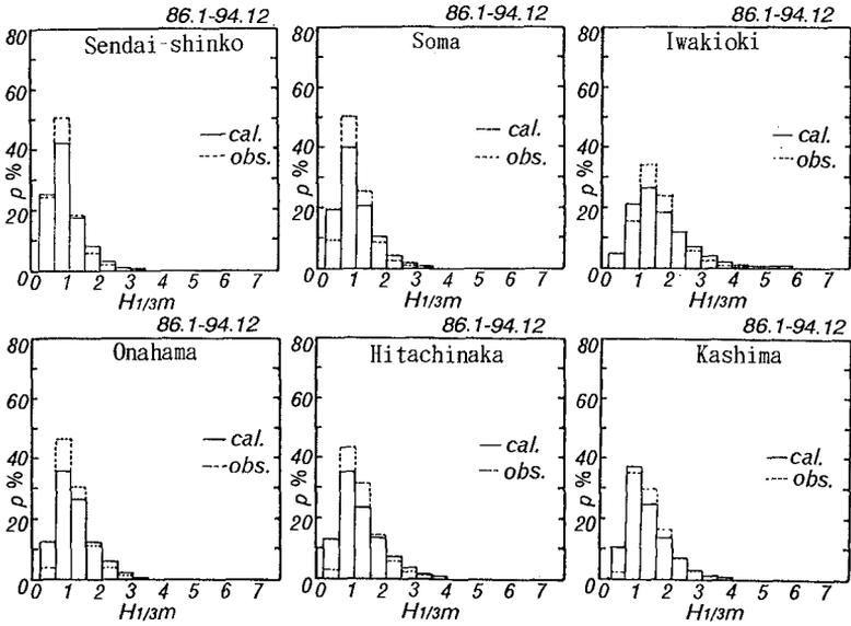
Figure 6. Comparison of Hindcast and Measurement for Histograms of Wave Height
