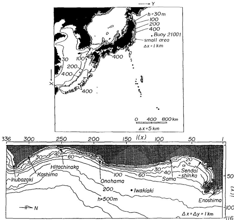
Figure 1. Medium and Fine Grid Systems of the Northwestern Pacific Ocean, Contour Plot of Water Depth and Location of Wave Hindcast Points
