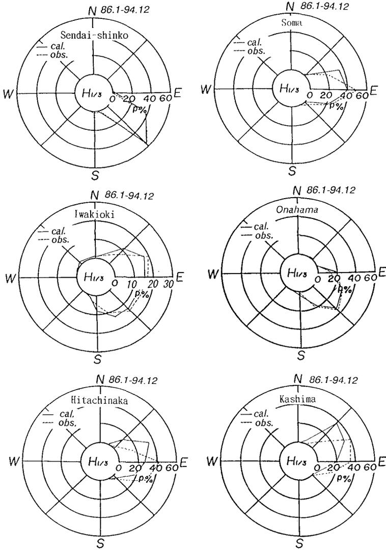
Figure 8. Comparison of Hindcast and Measurement for Directionally-Grouped Occurrence Rate of High Waves Exceeding 2 m
