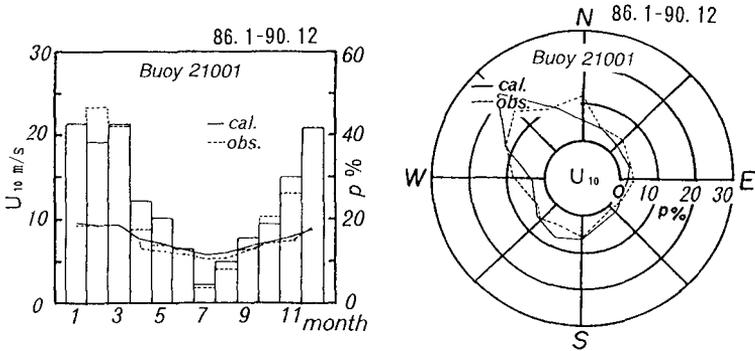
Figure 2. Comparison of Analysis Data and Measurement Data for Monthly-Variations of Mean Wind Speed and Occurrence Rate of Strong Winds, and Yearly-Average of Directionally-Grouped Occurrence Rate of Strong Winds
