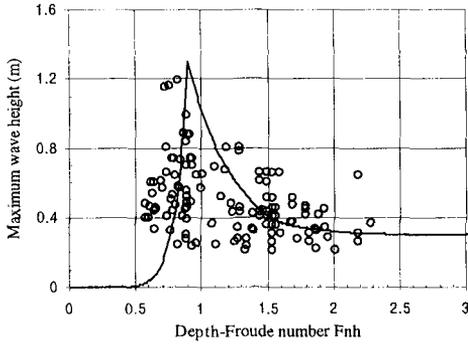
Figure 3. Maximum wave height of the long-periodic waves versus the depth-Froude number. The measured data (o o o) have been corrected to be valid in a distance of 700 m (~ 10 ship lengths) from the ship track. (—) indicates a trend line.
