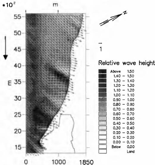
Figure 9. Wave propagation and transformation in Kalundborg Fjord, Denmark. The contour values show the relative wave height defined as the local wave height divided by the wave height at the boundary (the navigation route). The direction of the arrows indicates the wave propagation direction.
