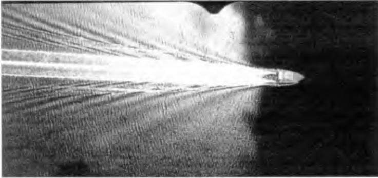
Figure 1. Aerial photograph of wave pattern generated at supercritical speed. The vessel speed is  $V_s = 35$  knots and the water depth is  $h = 13-14$  m. The Froude numbers are  $F_{nh} \sim 1.5$  and  $F_{nl} \sim 0.7$ . The overall length of the catamaran is approximately 78 m.
