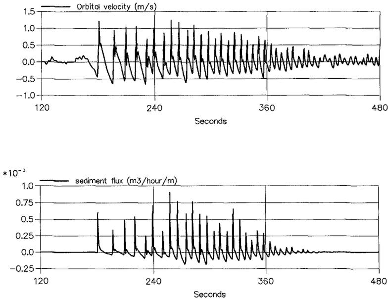
Figure 8. Time series of simulated wave orbital velocity (upper panel) and sediment flux (lower panel) caused by waves generated by a HSC. The water depth is 0.65 m.
