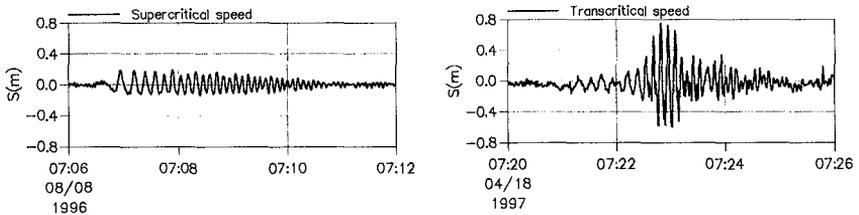
Figure 7. Time series of measured surface elevation in shallow water. Left panel shows the wake wash caused by an HSC operating in the supercritical speed range and the right panel for a transcritical speed. The water depth and distance to the navigation track are 2.4 m and 1500 m (left panel) and 3.2 m and 1100 m (right panel).
