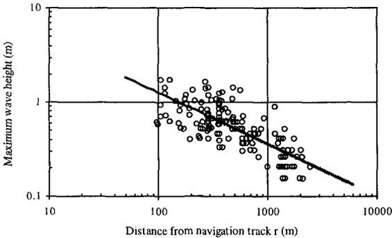
Figure 4. Maximum wave height of the long-periodic waves versus the distance from the ship track. The measured data (o o o) have been based on various field campaigns involving catamarans only. The trend line (—) is given by  $H_{max} = 16r^{-0.55}$ , where  $r$  (in meters) denotes the distance from the track.
