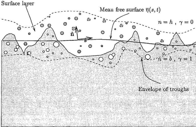
Figure 3: Global geometry adopted in the model for the surface layer.
