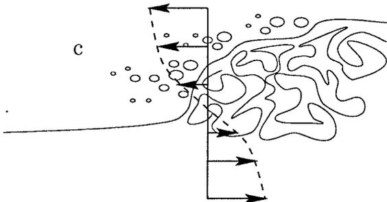
Figure 7: Sketch of the flow and of the velocity profile at the toe of a breaker propagating with celerity  $c$ .
