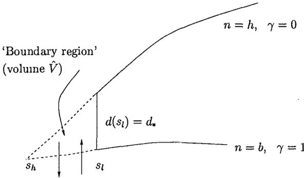
Figure 8: Sketch of the flow properties used in the modelling of the toe of the breaker.
