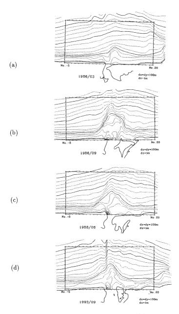
Fig. 3: Bathymetric charts at various stages.(a): March, 1986,(b): September 1986,(c): August 1988,(d): September 1993.
