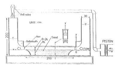
Fig.1 Schematical view of the U-shape tube
