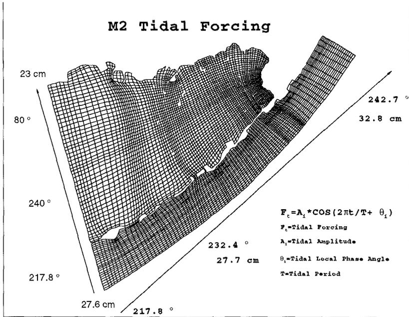
**Figure 6.** A model grid with 98x75 cells and open boundary conditions for M<sub>2</sub> tide in Florida Bay.
