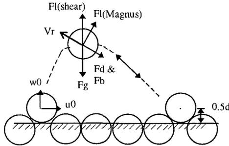
Figure 1 Force definition sketch of particle saltation
