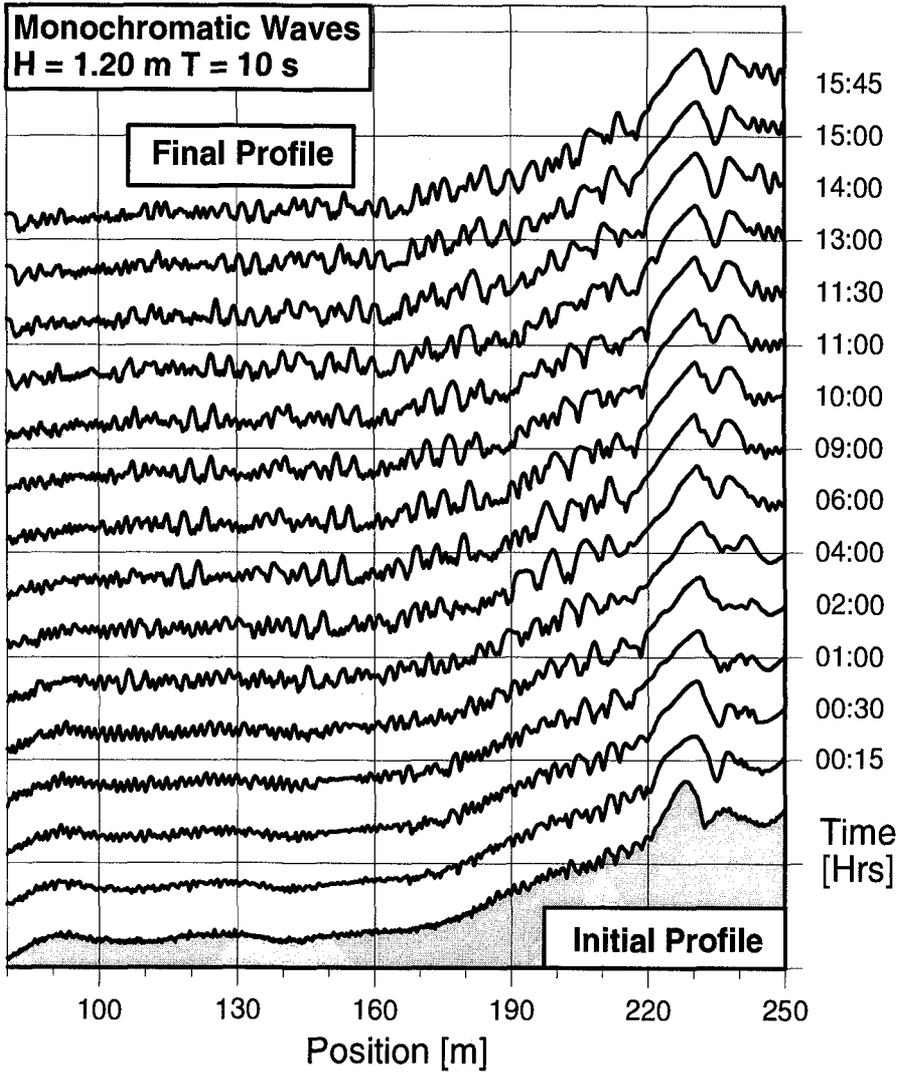
Figure 6. Development of bed forms during accretional wave conditions (Test Series 1).
