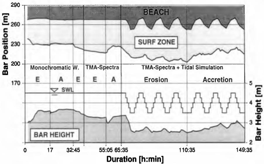
Figure 5. Definition of the surf zone (above) and position and height of bar over all Test Series' (below)
