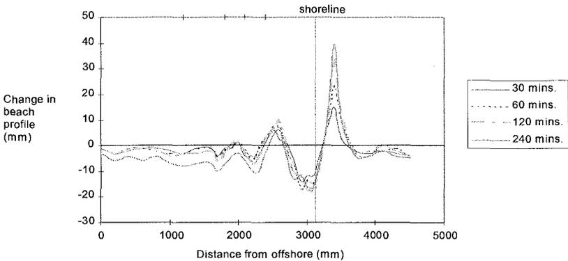
**Figure 6.** Change in bed elevation from original profile, case K.
