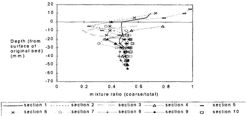
Figure 9c. Variation in mix ratio with depth at six cross-shore locations.
