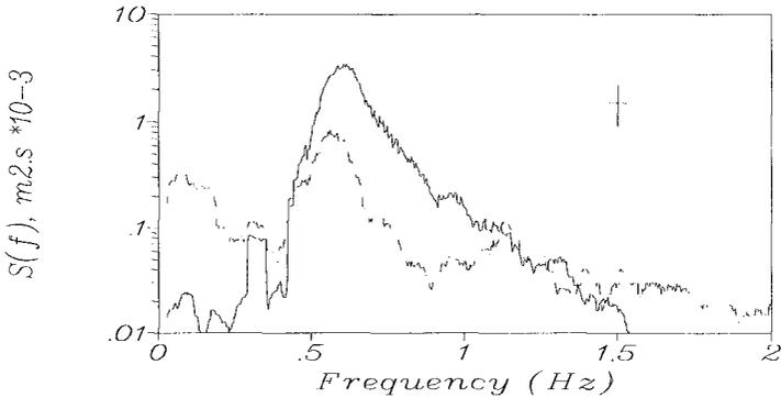
**Figure 2.** Wave spectra for case P outside the surf zone and close to the shoreline.
