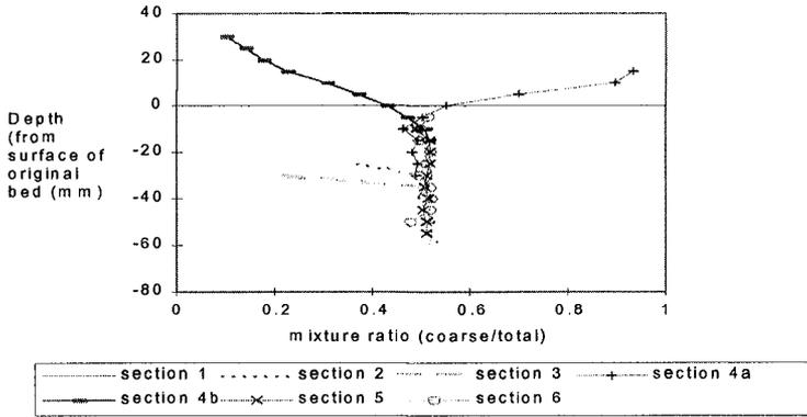
Figure 8c. Variation in mix ratio with depth at six cross-shore locations, case K.
