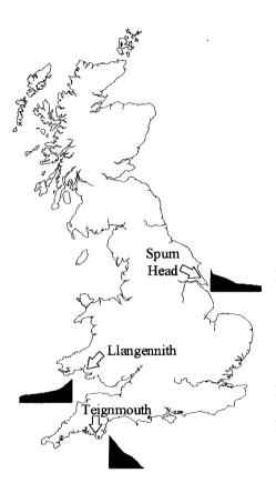
Llangennith: A dissipative high energy beach with a shallow beach gradient (0.014-0.020) with fine to medium quartz sands ( $D_{50}=0.21$ mm). This beach is west facing, has a tide range up to 9 metres, and broad surf (up to 350m) and intertidal (~ 500m) zones.
