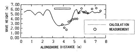
Fig. 5 Alongshore distribution of breaking wave height.
