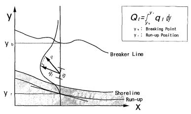
Fig. 4 Schematic illustration of the estimation method of the total longshore sediment transport rate by the cross-shore integration of the local sediment transport rate.
