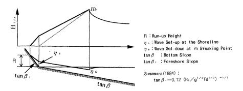
Fig. 3 Schematic illustration of the estimation method of the wave height and water level in the swash zone.
