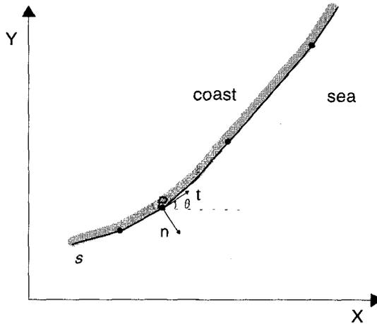
Figure 5. Curvilinear coordinate system.
