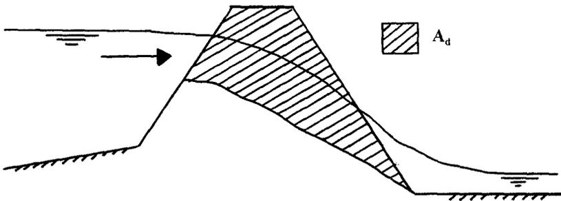
figure 6: definition of the eroded cross-section  $A_d$
