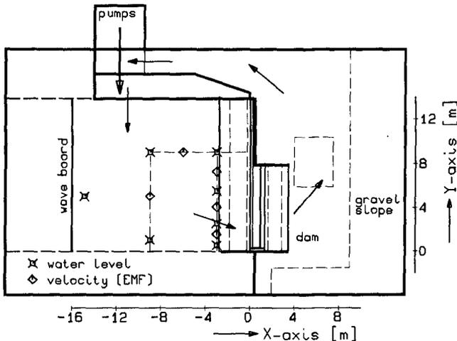
Figure 1: Planview of the wave basin lay-out
