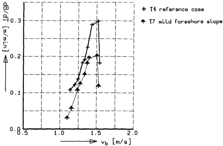
figure 5: development of the breach growth velocity as a function of the water velocity in the breach, shown is the effect of a mild foreshore slope
