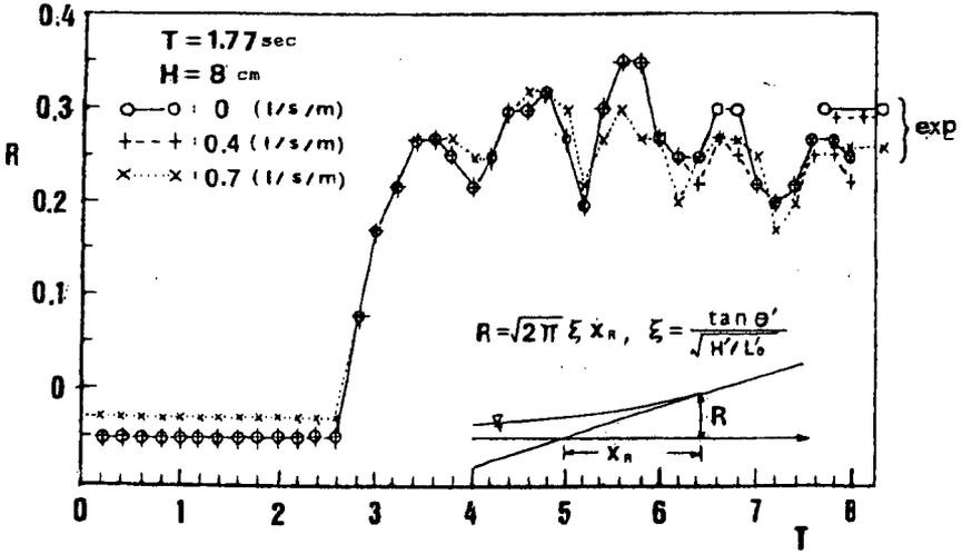
Figure 6 An example of measured and calculated runup
