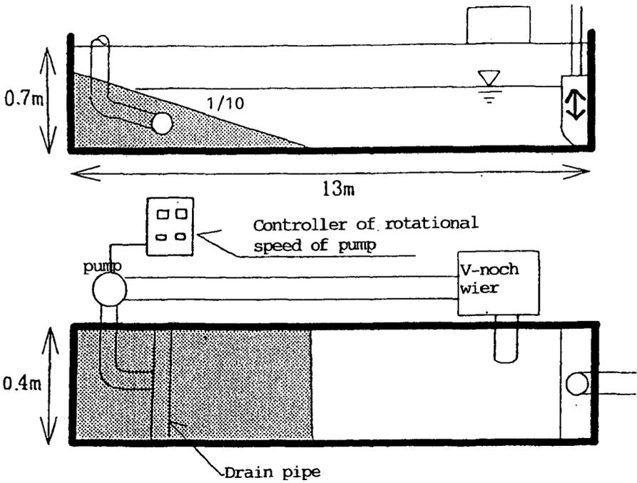
Figure 4 Experimental setup
