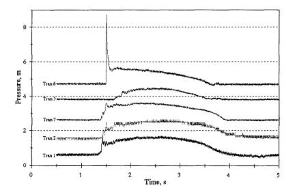
Figure 2: Typical pressure traces measured at prototype scale
