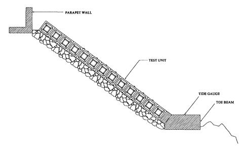
Figure 1: Typical cross-section of LaCollette Breakwater, Jersey, UK
