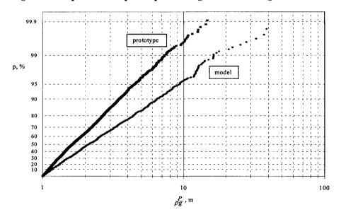
Figure 8: Comparison of pressure magnitudes using Froudian scaling
