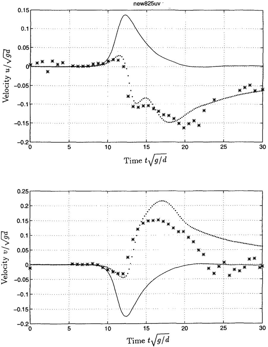
Figure 4: Comparison of particle velocity results from the present model, potential flow theory and experiment at  $x^* = 0.15$  and  $y^* = -0.825$  for solitary wave overtopping on breakwater C,  $H/d = 0.3$ ,  $d = 9in$ ;  $\cdots$  present model;  $—$  potential flow model;  $***$  experiment.
