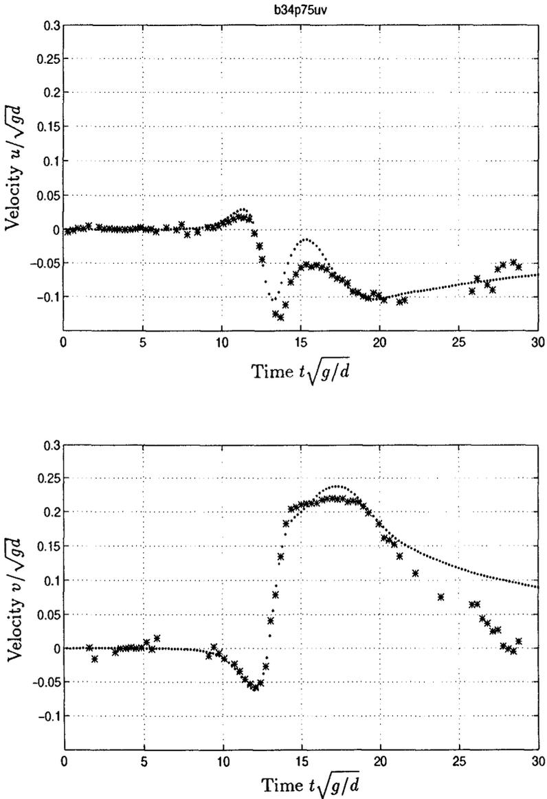
Figure 5: Comparison of particle velocity results from the present model and experiment at  $x^* = 0.15$  and  $y^* = -0.75$  for solitary wave overtopping on breakwater C.  $H/d=0.3$ ,  $d=9\text{in}$ ;  $\cdots$  present model;  $***$  experiment.
