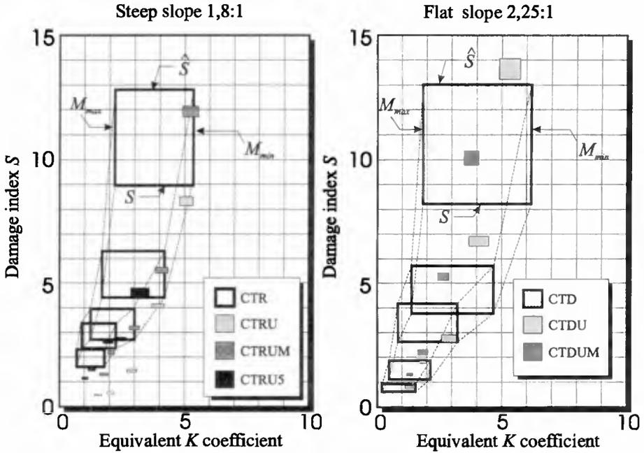
**Figure 9.** Comparison between graded and uniform material
