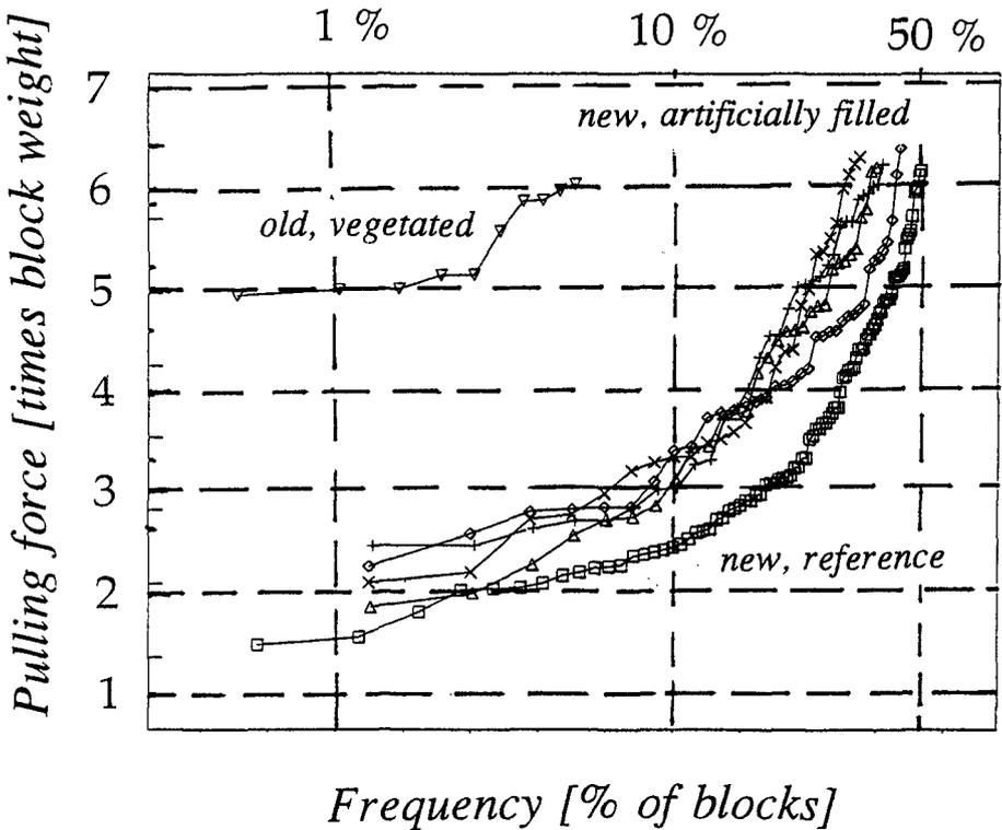
Figure 3 Results of pull out tests on test section
