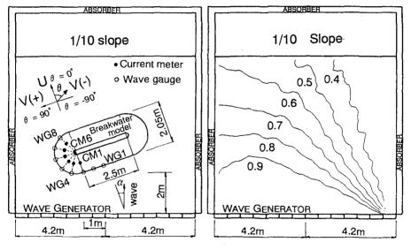
Figure 1 Plan view of the experimental set-up.
