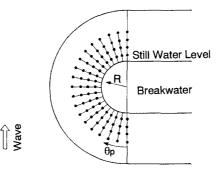
Figure 8 Measuring points of velocity components over the head.
