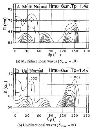
Figure 9 Spatial distribution of occurrence frequencies for armour stone movement.
