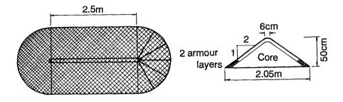
Figure 3 Plan and profile view of the breakwater model.
