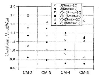
Figure 4 Comparison between U, V component velocities under 3D and 2D waves.
