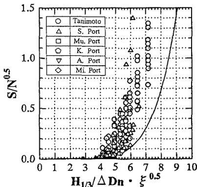
Figure 4 Relation between  $H_{1/3}/(\Delta Dn)\xi^{0.5}$  and  $S/N^{0.5}$
