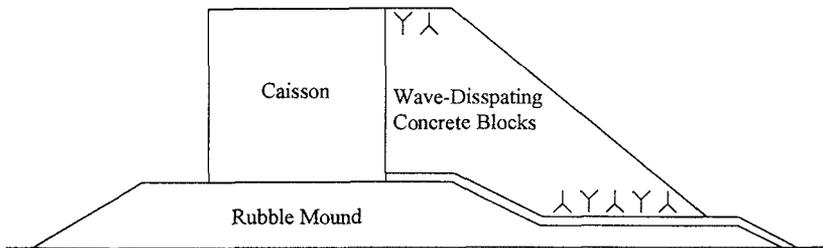
Figure 1 Typical cross section of horizontally composite breakwaters
