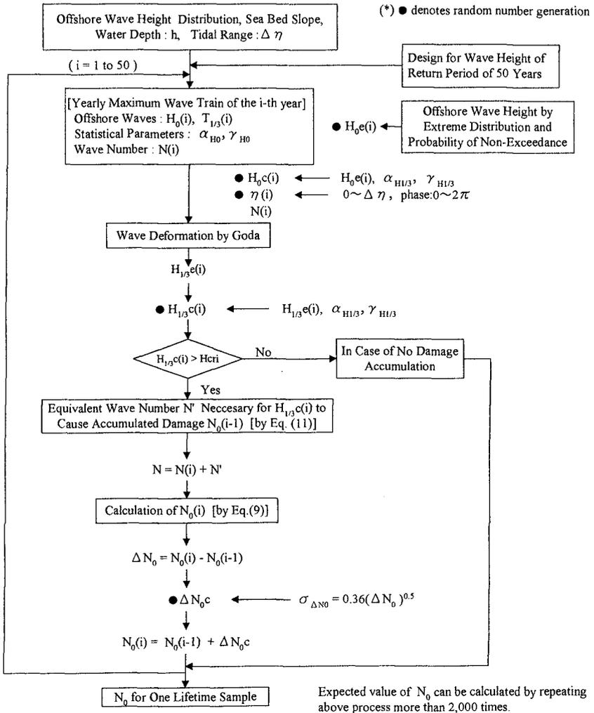
Figure 12 General calculation flow of one lifetime sample
