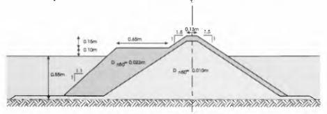
Figure 2: Initial profile for tests at DHI.
