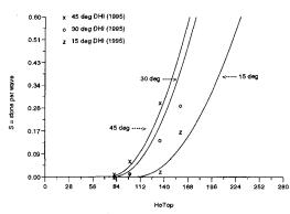
Figure 7: Longshore transport, in form of stone per wave, S, as function of  $H_o T_{op}$ .
