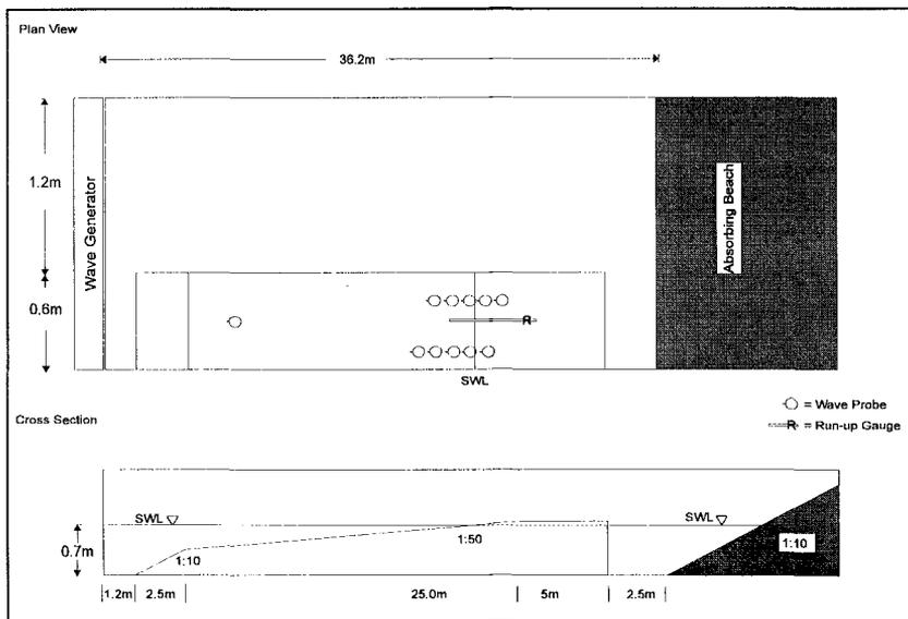
**Figure 1 Experimental Setup at QUCERL**
