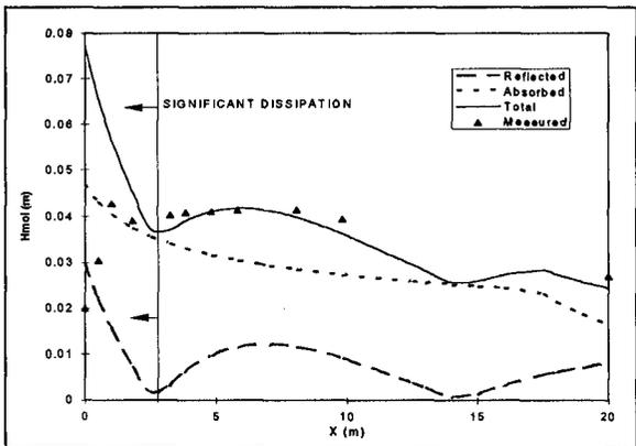
Figure 8 Example Model Results for Irregular Wave Test
