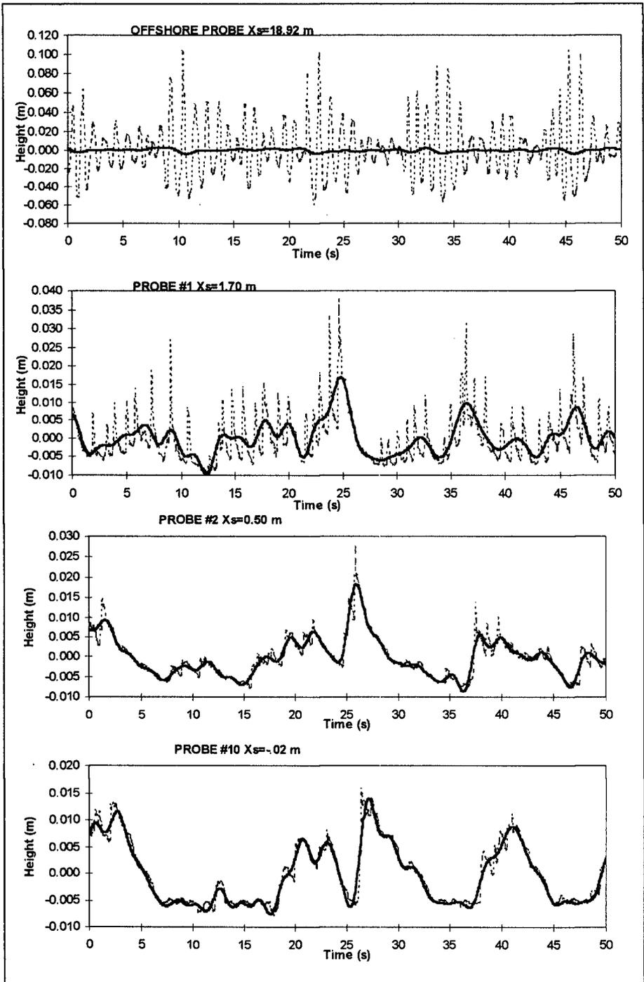
Figure 2 Example Wave Trains with Low-Pass Filtering
