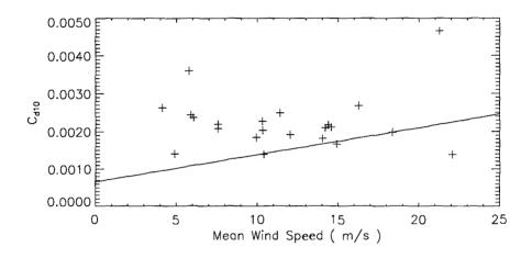
Figure 6: Drag coefficient estimates against wind speed during the typhoon.
