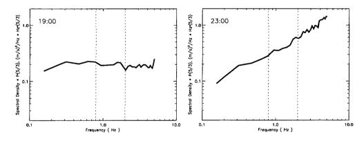
Figure 5: Wind Spectra  $S(f)f^{5/3}$  at 19:00 and 23:00, 29 Sep 94 (T9426)
