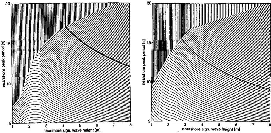
Fig. 8. Contours of run-up reliability function  $z$  as function of nearshore significant wave height and nearshore peak wave period for sea level 3.0 m (left) and 5.0 m (right) at Pettemer Zeewering (ref. de Valk 1996).
