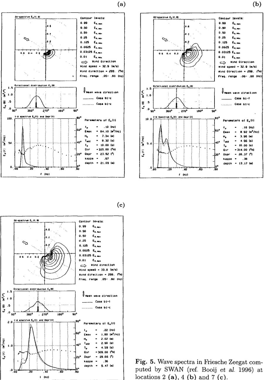
Fig. 5. Wave spectra in Friesche Zeegat computed by SWAN (ref. Booij et al. 1996) at locations 2 (a), 4 (b) and 7 (c).
