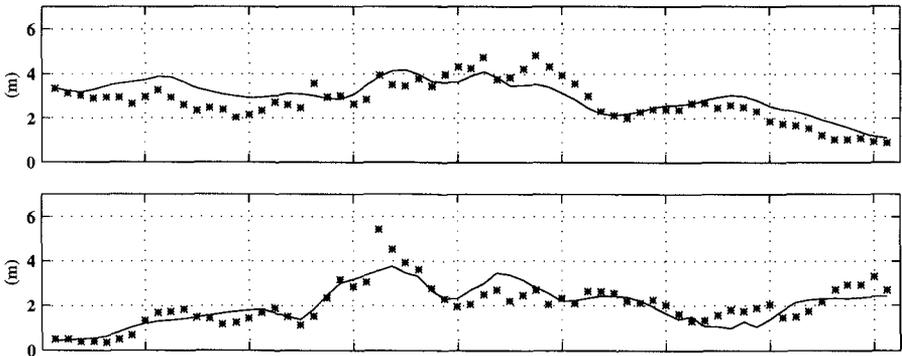
Fig. 7. Comparison between modelled (solid line) and recorded at EUR station (stars) time series of significant wave height for storm periods 15–22 Jan, 1983 (top) and 11–18 Feb, 1989 (bottom).
