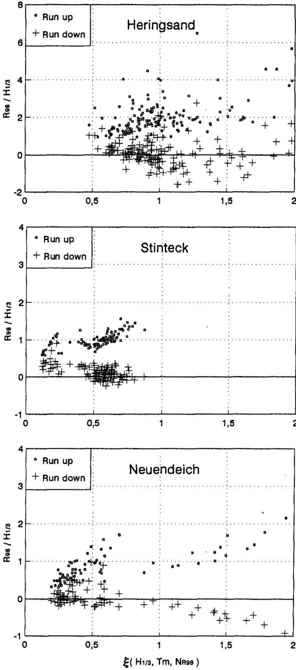
Fig. 15  $R_{98} / H_{1/3}$  versus breakerindex  $\xi$
