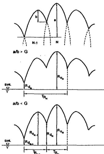
Fig. 11 Mode for separating of single run-up events
