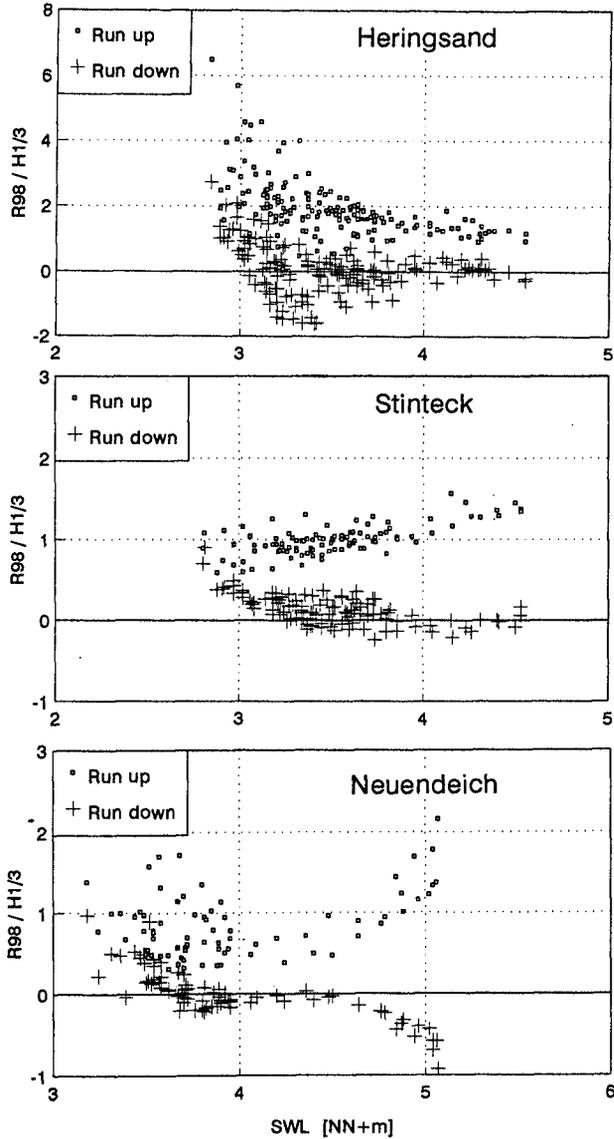
Fig. 13  $R_{98} / H_{1/3}$  versus stillwaterlevel  $SWL$
