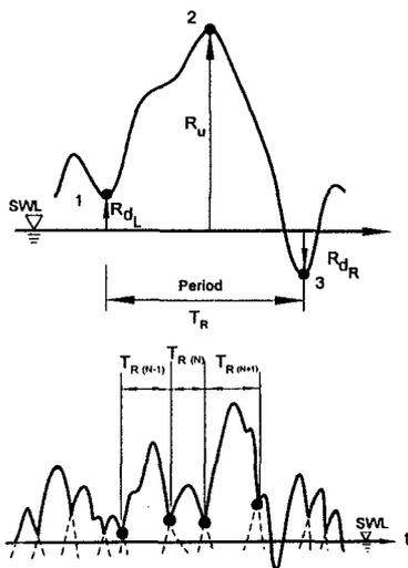
Fig. 10 Definition of run-up and run-down parameters
