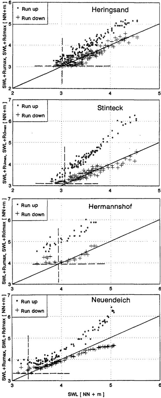
Fig. 12 Maximum run-up and run-down levels versus stillwaterlevels
