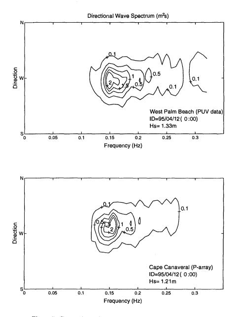
Figure 7: Comparison of analyzed directional wave spectra.
