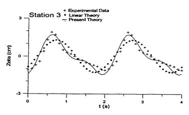
Fig. 3 Comparison of present numerical solutions with experimental results (Beji and Battjes, 1993), station 3
