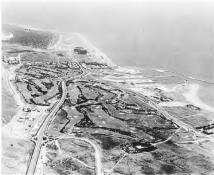
Fig 1. A View of the Effect Caused by the Littoral Drift Interruption. (Almerimar Marina, Almerian Coast)
