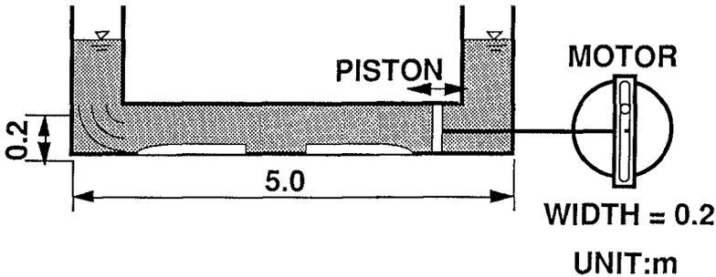
**Fig.2** U-shape oscillating water tunnel
