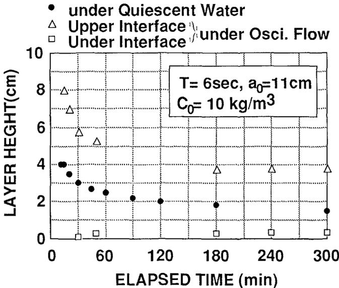
Fig.3 Temporal changes of the interface in height
