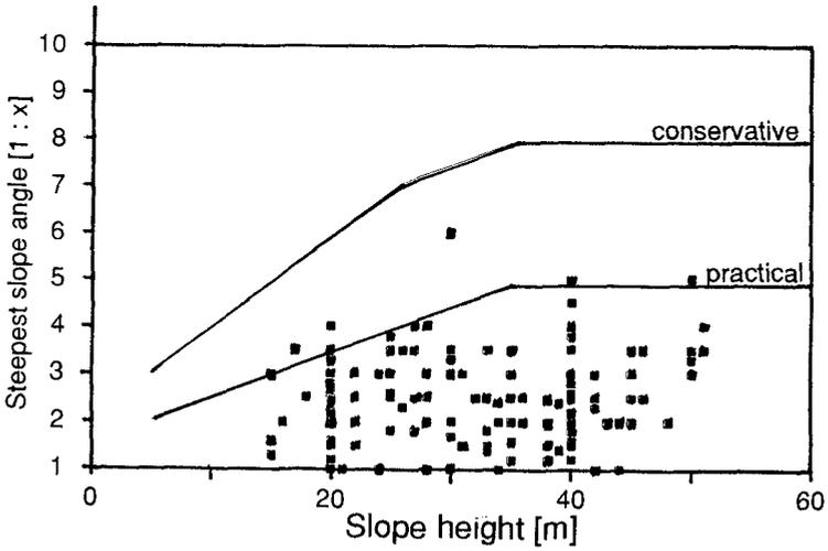
Figure 3 Actual flow slides compared to model results: Slope angle of steepest part of the slope as a function of slope height
