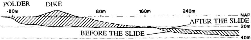
Figure 1 Example of an actual flow slide along the shore of the Eastern Scheldt basin (Leendert Abrahamspolder)
