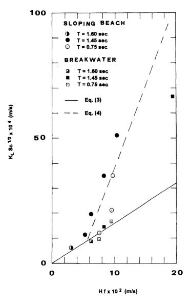
Fig. 5. Variation of the transfer coefficients with the wave parameter Hf.
