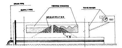
Fig. 2. Longitudinal view of the wave channel with the rubble mound breakwater.
