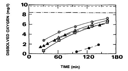
Fig. 4. D.O. - time histories for waves (incipient wave: H=7.1 cm, T=0.75 sec) breaking (i) on a sloping beach (open symbols) and (ii) on a breakwater (solid triangles refer to the concentration in front and solid circles to the concentration behind the breakwater).
