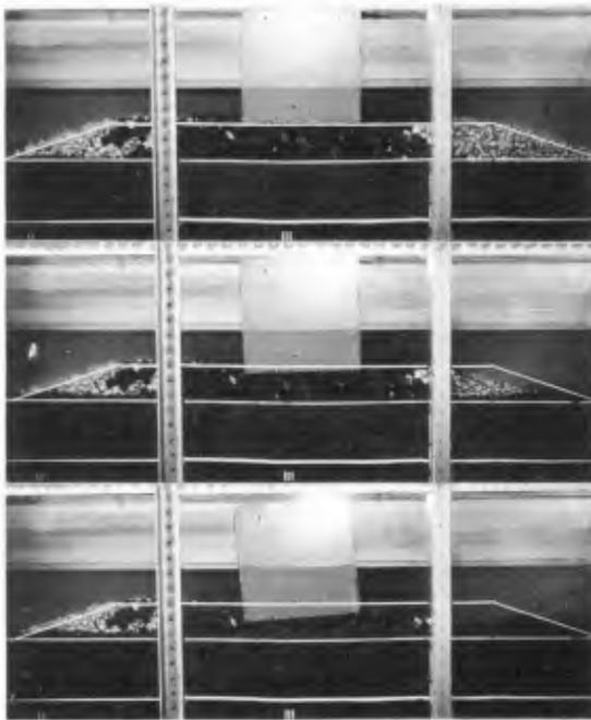
Fig. 7 Settlement of a Caisson Breakwater
